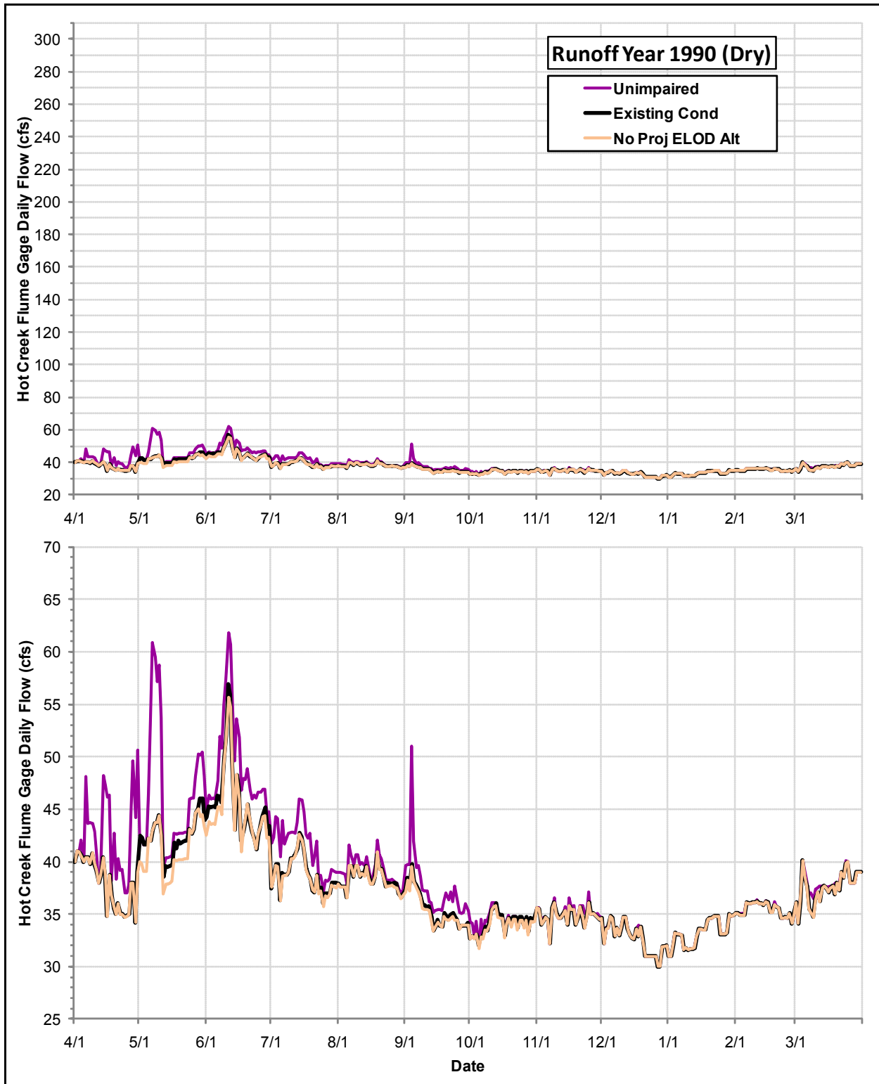
Daily Flows (cfs) at the USGS Hot Creek Flume Gage under the No Project Alternative (Existing Level of Demand), the Existing Condition and the Index of Unimpaired Conditions during Runoff Year 1990
