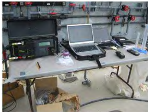
Figure 1: Fluorometer and Data Collection Setup
